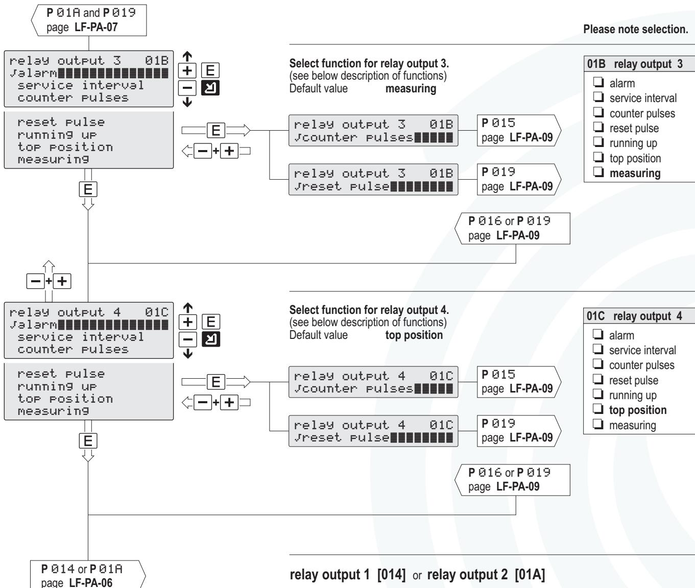
**relay output 1 [014] or relay output 2 [01A]**
